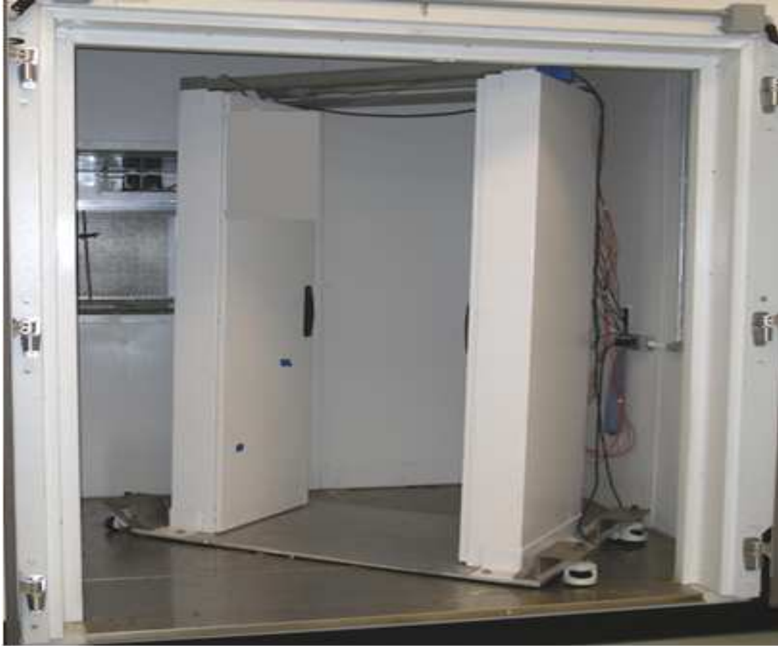
Figure 3.2: Pedestrian RPM placed inside the Tenney Environmental Chamber.
